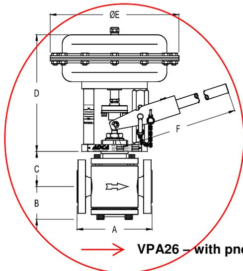
→ VPA26 – with pneumatic actuator and manual operation
